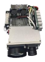
This LTD employs an LDA-pumped Nd:YAG crystal combined with an electro-optic Q-switching technology, to achieve a typical 1064nm pulsed laser output with a single pulse energy of 60mJ, and a beam divergence angle of 0.3mrad.
