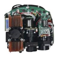
It employs an LDA-pumped Nd:YAG crystal combined with an electro-optic Q-switching technology, to achieve a typical 1064nm pulsed laser output with a single pulse energy of 45mJ, and a beam divergence angle of 0.5mrad.
